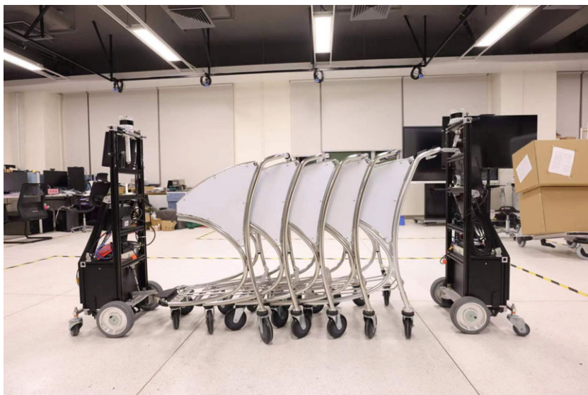
Figure 1. The luggage trolley transportation system.
