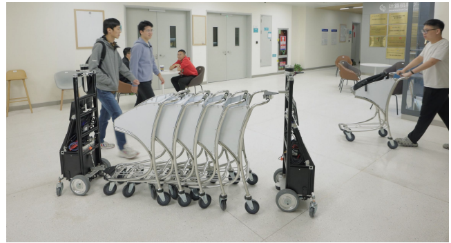
Fig. 1. A snapshot showing a dual-robot system transporting a series of luggage trolleys in tandem in a dynamic environment.
